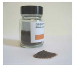
The spherical nature of Pt(0) EnCat<sup>™</sup> makes it ideally suited to continuous flow processes or batch methodologies
